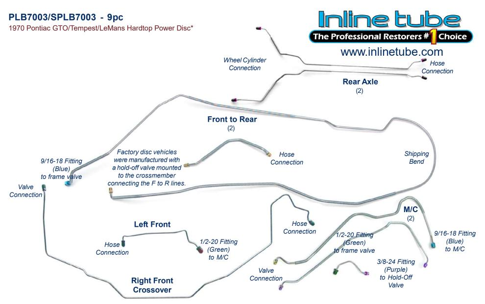
\*Reproduction of factory brake lines for unmodified vehicles using original components. This system has a hold-off valve at the M/C with 3/8-24 fittings and a frame distribution block and rear hold-off valve that must be re-used, or available from Inline Tube (PR115, PR104D, PR107). The Front to Rear uses a 9/16-18 fitting at the valve. Images are for identification purposes and are not to scale.
