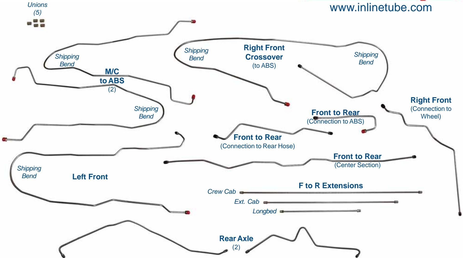
\*Re-designed for easier shipping/installation of factory brake lines for unmodified vehicles using original components. Specific applications may not require all pieces provided.
