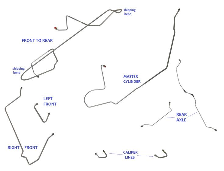
\*Re-designed for easier shipping/installation of factory brake lines for unmodified vehicles using original components.
