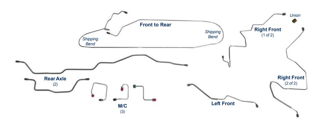
\*Re-designed for easier shipping/installation of factory brake lines for unmodified vehicles using original components.
