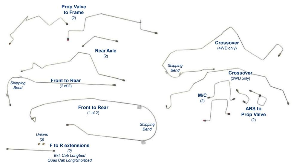
\*Re-designed for easier shipping/installation of factory brake lines for unmodified vehicles using original components.
