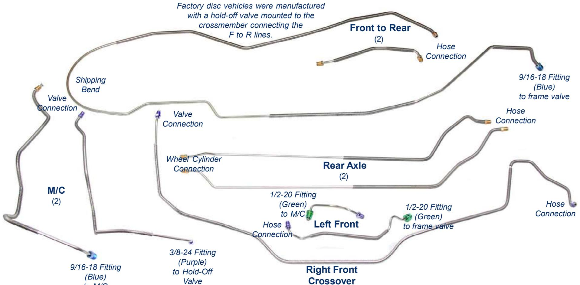
\*Reproduction of factory brake lines for unmodified vehicles using original components. This system has a hold-off valve at the M/C with 3/8-24 fittings and a frame distribution block and rear hold-off valve that must be re-used, or available from Inline Tube (PR115, PR104D, PR107).
