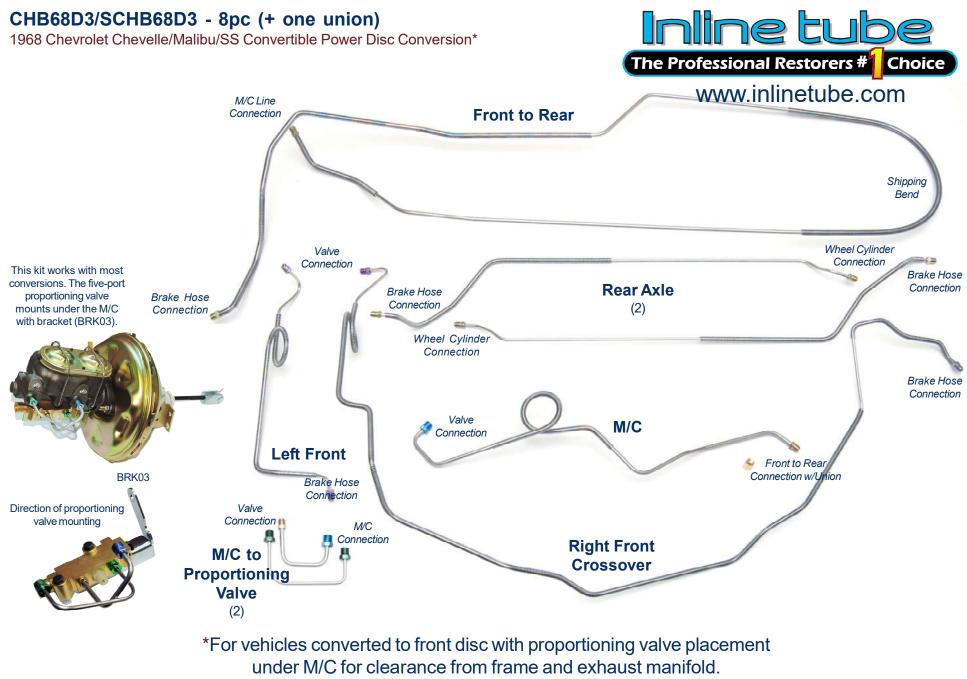
The correct proportioning valve bracket is Inline Tube part BRK03. Images are for identification purposes and are not to scale.
