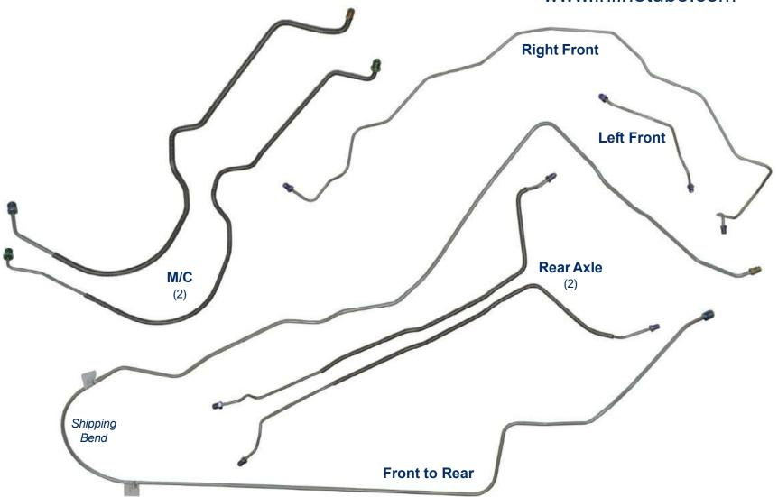
\*Reproduction of factory brake lines for unmodified vehicles using original components. *Images are for identification purposes and are not to scale.*
