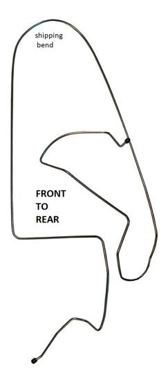
\*Re-designed for easier shipping/installation of factory brake lines for unmodified vehicles using original components.
