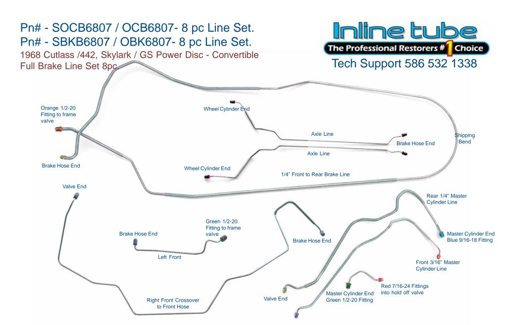
This is a factory brake line set for unmodified cars using original components. This braking system has a hold off valve at the master cylinder with red 7/16-24 fittings and a frame distribution block that must be reused or are available new from inline tube. The front to rear brake line uses a orange 1/2-20 fitting at the valve. This is every hard line in the system.
