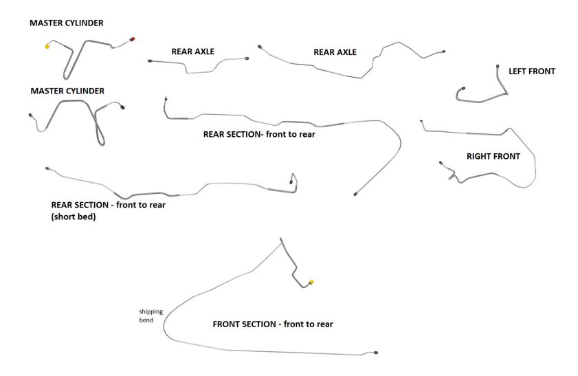
\*Re-designed for easier shipping/installation of factory brake lines for unmodified vehicles using original components.
