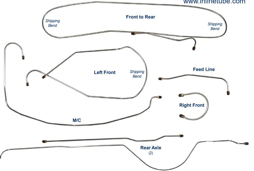
\*Reproduction of factory brake lines for unmodified vehicles using original components. Images are for identification purposes and are not to scale.
