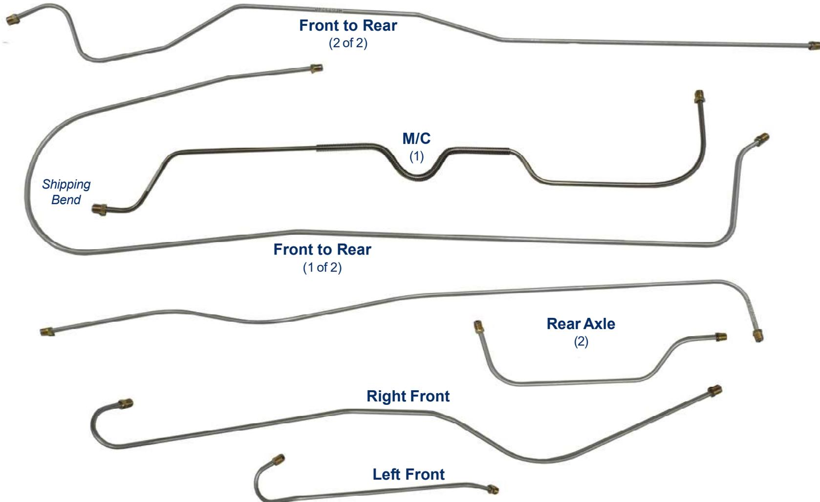
\*Reproduction of factory brake lines for unmodified vehicles using original components.
