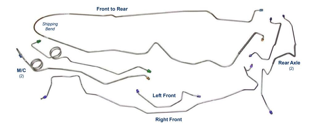
\*Reproduction of factory brake lines for unmodified vehicles using original components. Images are for identification purposes and are not to scale.
