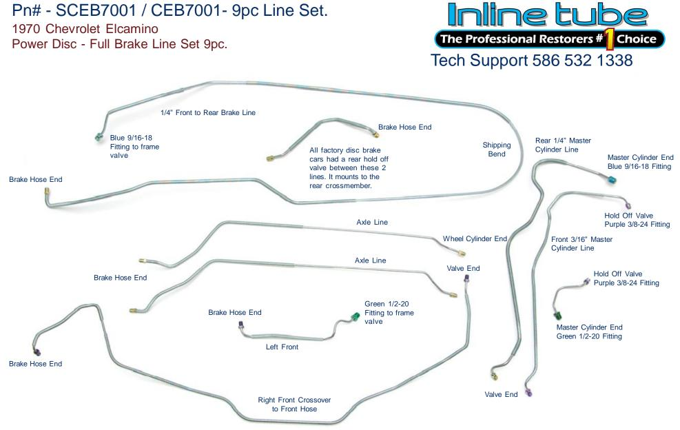
This is a factory brake line set for unmodified cars using original components. This braking system has a hold off valve at the master cylinder with Purple 3/8-24 fittings and a frame distribution block and a rear hold off valve that must be reused or are available new from inline tube. The front to rear brake line uses a blue 9/16-18 fitting at the frame valve. This is every hard line in the system.
